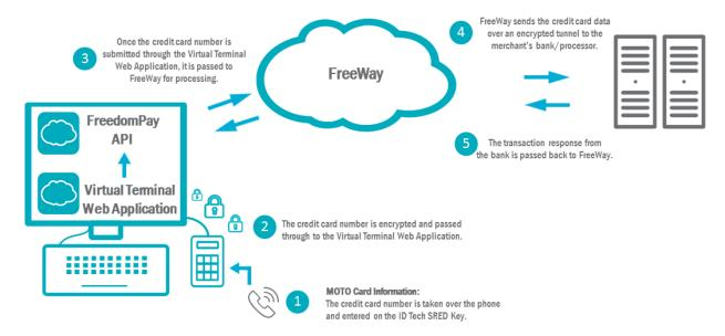
SREDKey data captured by a call center (top diagram) can be sent to FreedomPay's cloud-based processing platform, then forwarded to the merchant's bank for clearing. From the moment of capture, sensitive cardholder data is encrypted. When used in a Virtual Terminal environment (lower diagram), SREDKey can keep the merchant out of PCI scope, since keystrokes are not captured in the clear but are encrypted at the moment of key entry, before reaching the merchant's computer. (Source: FreedomPay)
